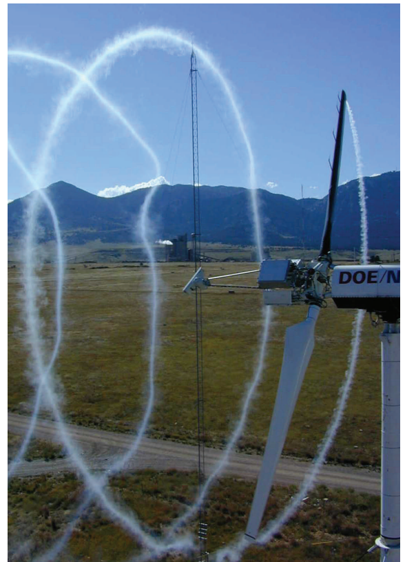
Wind Turbine Tip Speed Visualization using smoke at the National Renewable Energy Laboratory (NREL).
