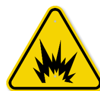
Risk of explosion
